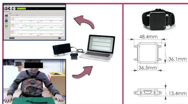
Figure 1. Experimental setup: the 5 sensing units (SUs) are attached to the body at predefined spots and data are collected and visualized via the developed software interface.
