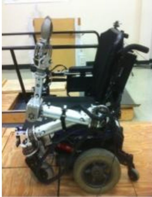
Figure 9 Reflective Markers and IMUs on WMRA
