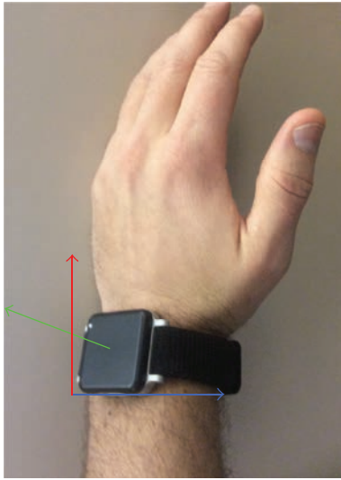
Figure 1: Inertial measurement unit on the left wrist. Blue arrow, x -axis. Red arrow, y -axis. Green arrow, z -axis.
