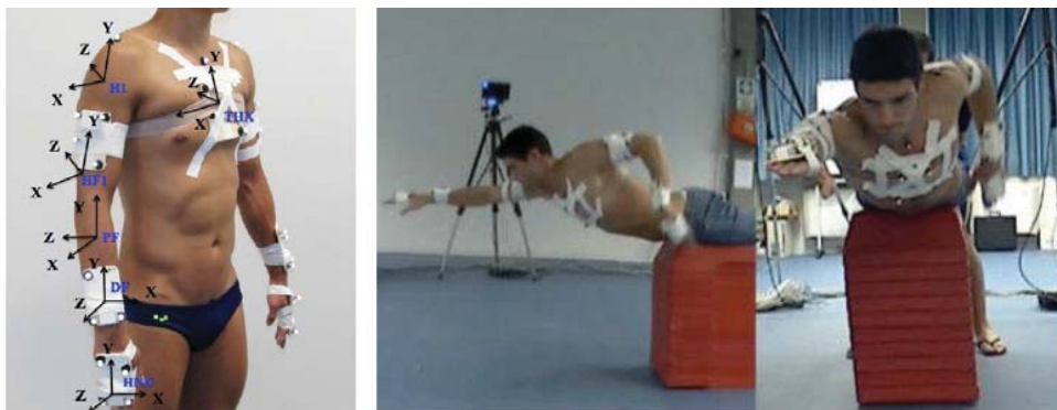
Figure 1. Left: inertial and IMMUs positioning on body segments detailing the anatomical system of reference axes. Right: lateral and anterior views during front crawl simulation.
