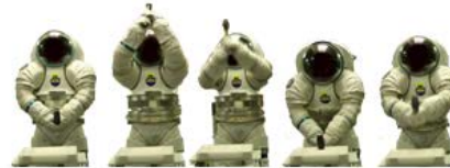
Figure 6. Space suit movement tasks performed by each subject. Three isolated joint tasks are performed: Elbow Flexion/Extension, Shoulder Flexion/Extension, and Shoulder Abduction/Adduction . Two functional tasks were performed: Cross Body Reach and Overhead Hammering . Subjects were given very specific instructions on how to perform the isolated joint tasks, while subjects were given way-point markers to meet and allowed to develop their own biomechanical strategies for the functional tasks. Subject in Mark III suit is shown.
