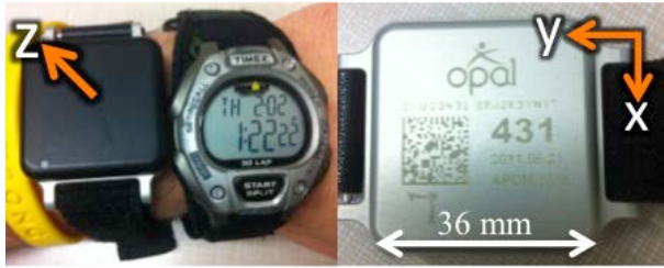
Fig. 1: APDM IMUs are small wearable devices. Axes are shown for IMU body reference frame.
