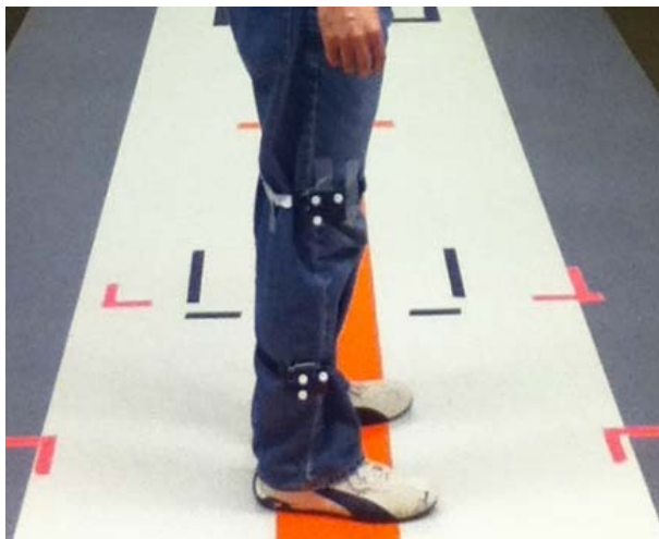
Fig. 2: IMU placement and reflective marker locations.
