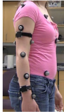
Fig. 2. Reflective markers and Opal inertial sensors (APDM, Inc.) placement on the arm of one of the subjects.
